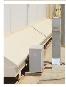
Motorized rack and pinion gear system for remote operation.
